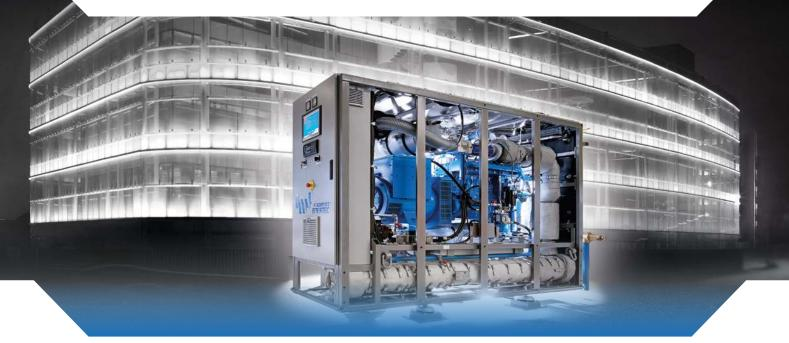
Our ENERGIN® CHP units are compact cogeneration plants with highly efficient heat recovery from the jacket water and the exhaust gas of the gas engine. The innovative design allows an easy and space-saving installation. All major components like gas engine generator unit, heat exchangers, circulation pumps, primary exhaust silencer and control cabinet are factory mounted on a common frame.
